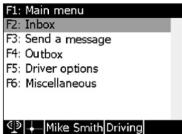
The availability of items on the *Main Menu* are access controlled. It is possible to configure the MDT 860 to display any of the items above. This configuration will be possible over the air from the OnlineAVL application or locally via the Configuration menu. Refer to section 8.9 *Main Menu*.
